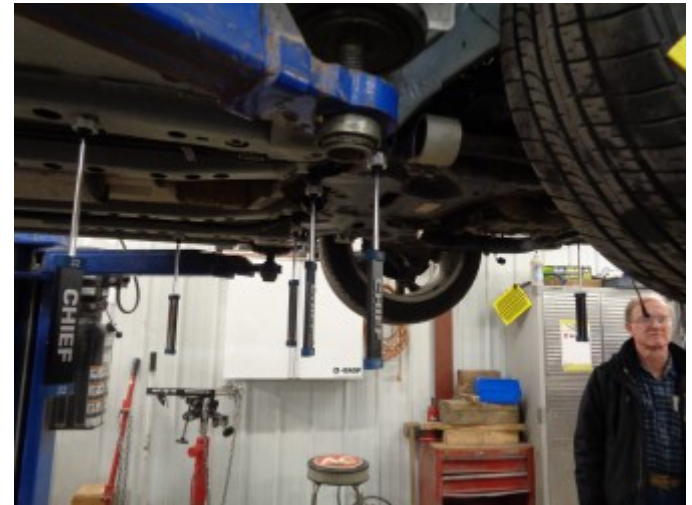
Vehicles are inspected using a computer and laser to identify hidden structural damage
